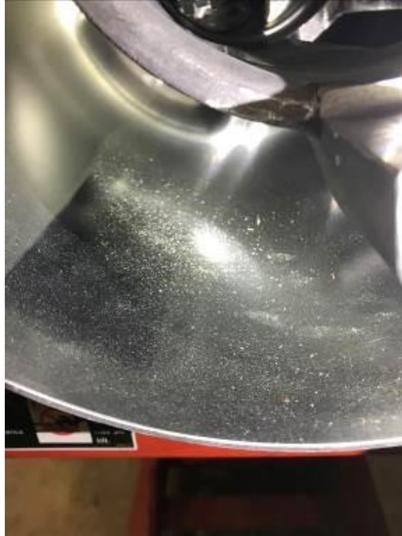
Figure 3: Metal Particles inside Exhaust Enclosure
